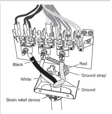
The neutral or ground wire of the power cord must be connected to the neutral terminal located in the center of the connector block. The power leads must be connected to the outside terminals.
